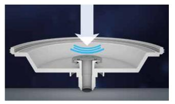
Oscillating non return valve, ensures that the non return valve is not blocked with any dirt.
