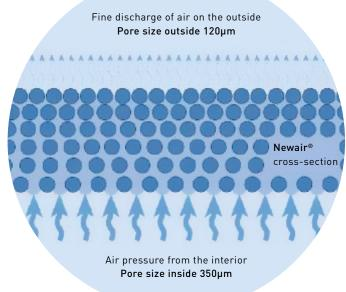
The newair aerator is characterized by a special material structure. The size of the pores reducing in flow direction. On the one hand there will be created a huge upstream flow area for the air, on the other hand there will be reached a fine allocation of the bubbles by a small pore size on the outlet side.
