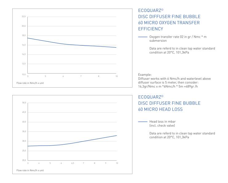
Comparable values can only be obtained with a similar setup and condition. Depending on the tank geometry, slit chart, water depth and planar allocation, the quoted values can change. All the data are based on clean water 20° temperature, 1013mbar / 68°F, 101,3kpa. All data are approximate data!
